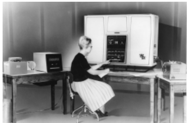
Fig. 5. The D2 prototype had a very small CPU module. It weighed some 200 kilos and needed only a 250-watt power supply. The emblem in the lower right corner was changed, depending on to whom it was shown: D2 for potential civilian customers and SANK (Saab’s Numeriska Kalkylator) for potential military ones.
