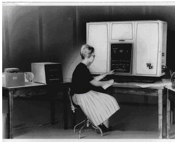
Figure 1. The prototype computer SANK-1 or SaabD2 with strip reader, punch, digital display and the operator. In operation from October 1960
